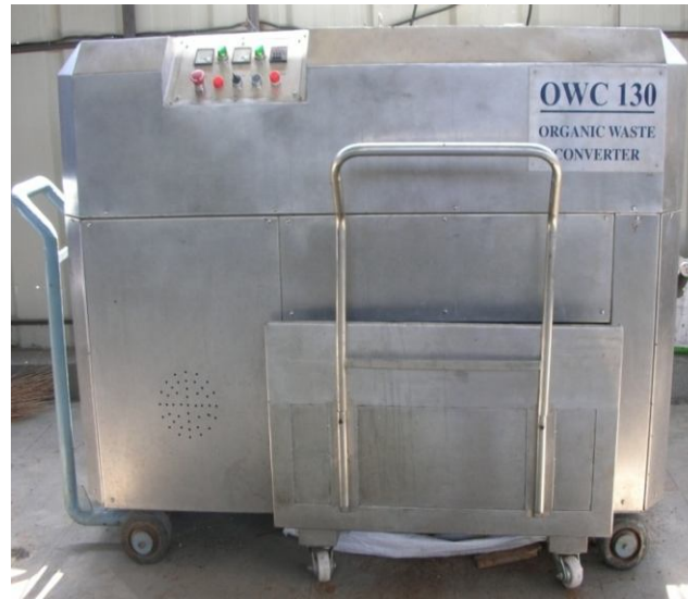
Waste batch size: 50kg Power: 8HP 3Phase
