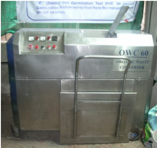
Waste batch size: 25kg Power: 4HP 3Phase
