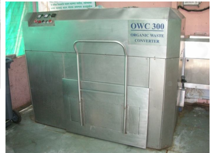
Waste batch size: 125kg Power: 13.5HP 3Phase
